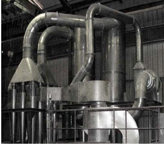
**Fig.7a –Sulphanilic acid cyclones**
