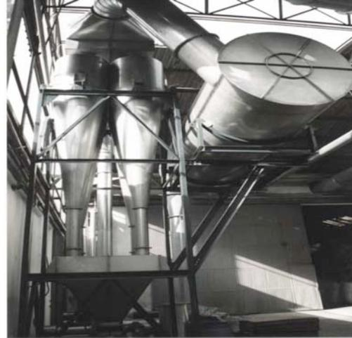
**Fig.7b –Corch waste boiler cyclones**
