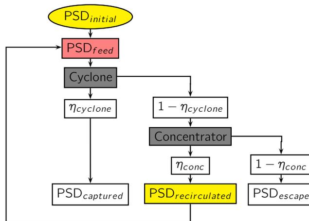
**Figure 2:** Iterative process concerning the processed particle size distribution
