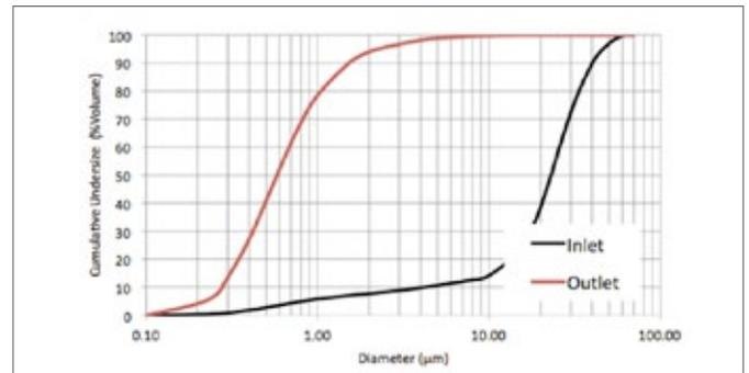
Fig. 3 - Particle size distribution used in simulations (Coulter)
