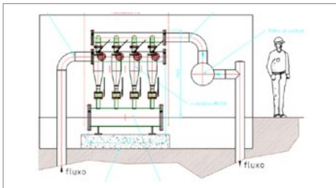
Fig.5 – General arrangement scheme | 4 Hurricane HR cyclones of Ø 200mm
